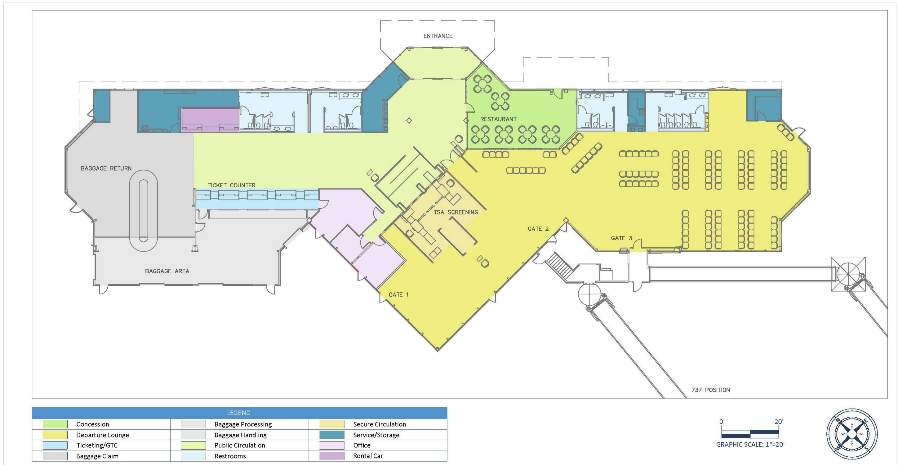
Exhibit 2-7- Terminal Building Floor Plan
